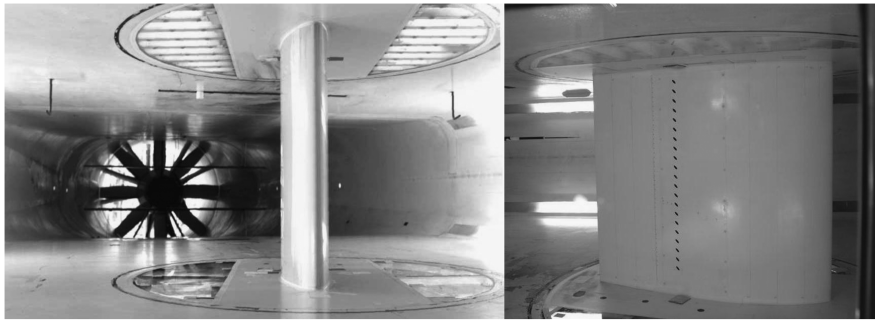
Fig. 10 Picture of the DU96 airfoil in the laminar wind tunnel.
